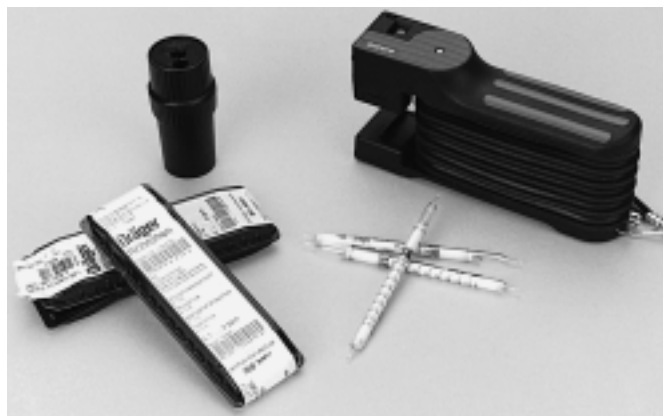
FIG. 6—Dräger Accuro® Pump and colorimetric tubes for the detection of phosphine gas.
